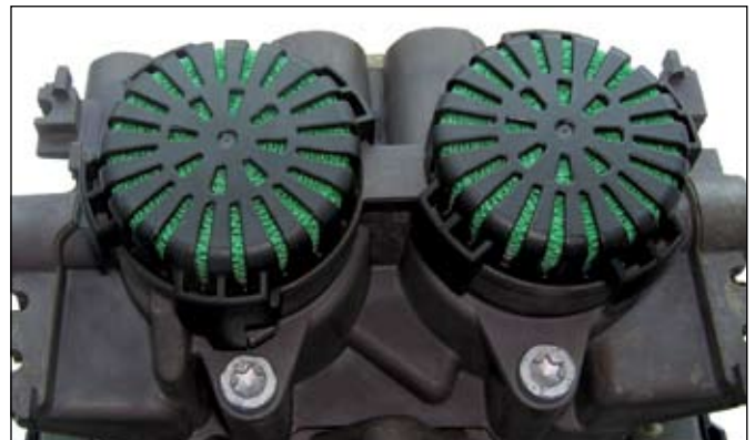
Fig. 8-3: Exhaust silencers on TEBS G2 Brake Module
