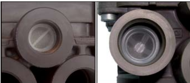
Fig. 8-1: Port filters in the TEBS G2 Brake Module (flat filter), left, and TEPM-S / EMS (conical filter), right
